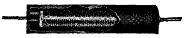
Cross Section—showing progressive interleaved windings for higher resistance values in less space.
